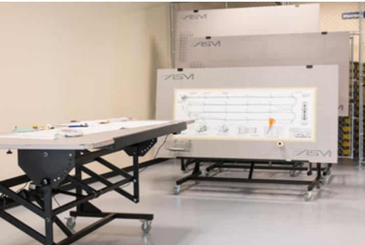
BOSTONtec wire harness board frames in multiple positions
